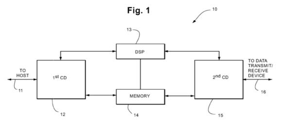
As shown in Figure 1 above, interface device 10 connects to a host device via host line 11, and to a data transmit/receive device via output line 16. *Id.* at 4:46–62. Interface device 10 includes first connecting device 12, second connecting device 15, digital signal processor 13, and memory
