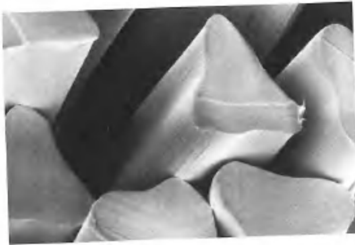
Figure 8.6 Photomicrographs of trilobal nylon.
