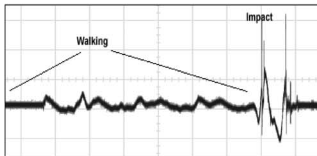
Fig. 10. Impact sensor output for walking and a fall
