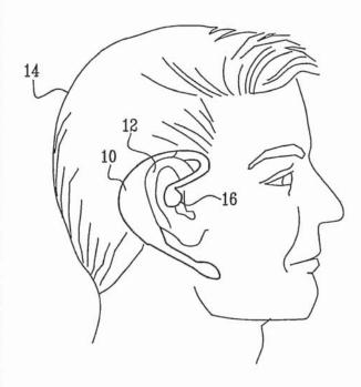
(57) Abstract: A physiological monitoring device (10) includes a device housing (11) shaped to fit behind an ear (12) of a subject and a sensor (18, 28, 30) attached to the device housing so as to sense a physiological characteristic of the subject at a location behind the ear. An earphone speaker (16) extends from the device housing towards an ear canal of the subject and provides an audible communication to the subject responsively to the physiological characteristic.
