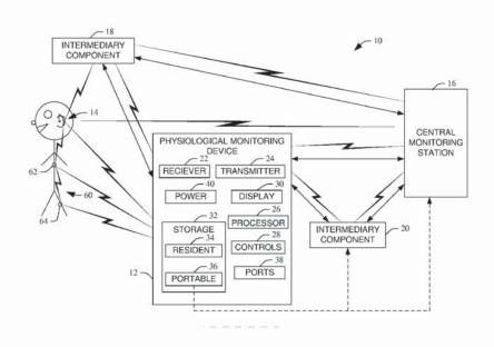
(57) Abstract: A portable physiological monitoring device (12) includes a receiver (22) that wirelessly receives physiological measurements from each of a plurality of in-the-ear probes (14) upon entering a communication range of one of the in-the-ear probes (14). The portable physiological monitoring device (12) farther includes a display (30) for presenting the physiological measurements.
