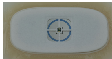
Fig. 5. The assembled patch with a pulse oximetry sensor made as a concentric photodiode around two LEDs placed in the center. The little square frame around the LEDs is to prevent light going directly from the LEDs into the photodiode.
