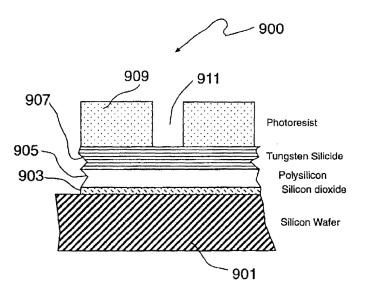
Figure 9 depicts substrate 901 having a stack of layers including oxide layer 903, polysilicon layer 905, tungsten silicide layer 907, and photoresist masking layer 909 with opening 911, from the treatment method shown in Figure 10, reproduced below. Ex. 1001, 17:58–18:57.
