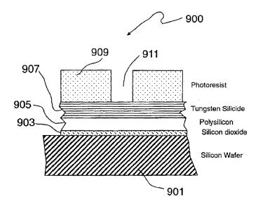
Figure 9 depicts substrate 901 having a stack of layers including oxide layer 903, polysilicon layer 905, tungsten silicide layer 907, and photoresist masking layer 909 with opening 911, from the treatment method shown in Figure 10, reproduced below. *Id.* at 17:58–18:57.
