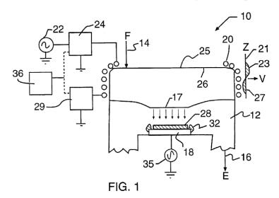
Figure 1 depicts a substrate (product 28, such as a wafer to be etched) on a substrate holder (product support chuck or pedestal 18) in a chamber
