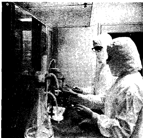
FIG. 22-8. Aseptic filling of vials with liquid under vertical laminar airflow, followed by stoppering with forceps by hand. (Courtesy of University of Tennessee.)
