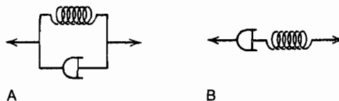
FIG. 6-20. Spring and dashpot representation of viscoelastic elements. The Kelvin element (A) has the components in parallel position, whereas the Maxwell element (B) has them in series.
