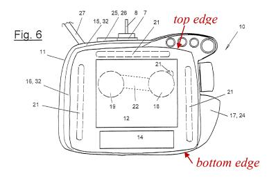
17. Wörn col. 2, line 65 – col. 3, line 2, states: "One or more switching keys, which are designed as, e.g., permission and/or start/stop keys, are located on the underside of the housing in the vicinity of the grip strips in a position favorable for gripping." Wörn col. 5, lines 63-65 states: "Switching keys (21), which are preferably arranged in the area of the recessed grip (31), are located at one or more
