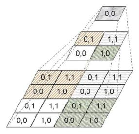
The diagram above depicts how the highest resolution tiles loaded by TerraCutter contribute to the pixels at lower resolution. We refer to the tiles loaded by the TerraCutter program as the "base scale" or "base tiles".
