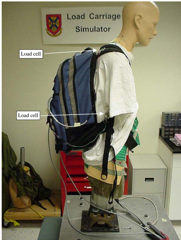
Fig. 1. Load carriage simulator used for data collection (tight shoulder straps configuration shown).
