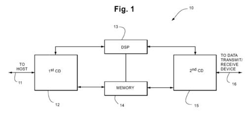
As shown in Figure 1 above, interface device 10 connects to a host device via host line 11, and to a data transmit/receive device via output line 16. *Id.* at 5:47–63. Interface device 10 includes first connecting device 12, second connecting device 15, digital signal processor 13, and memory means 14. *Id.* In a preferred embodiment, the interface device is
