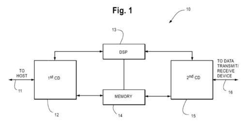
As shown in Figure 1 above, interface device 10 connects to a host device via host line 11, and to a data transmit/receive device via output
