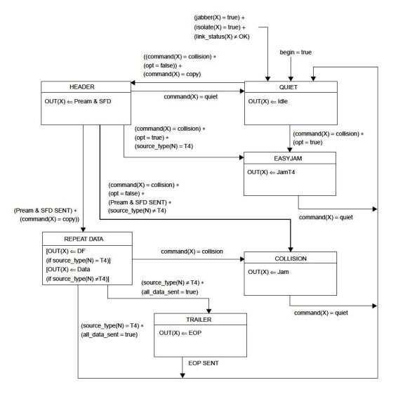
Figure 27-5—100BASE-T4 transmit state diagram for port X
