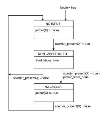
Figure 27-7—Receive timer state diagram for port X
