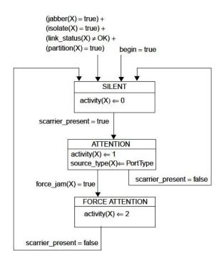
Figure 27-3—Receive state diagram for port X
