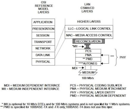
\*\*\* AUTONEG communicates with the PMA subayer through the PMA service interface messages PMA\_LINK.request and PMA\_LINK.indicate
