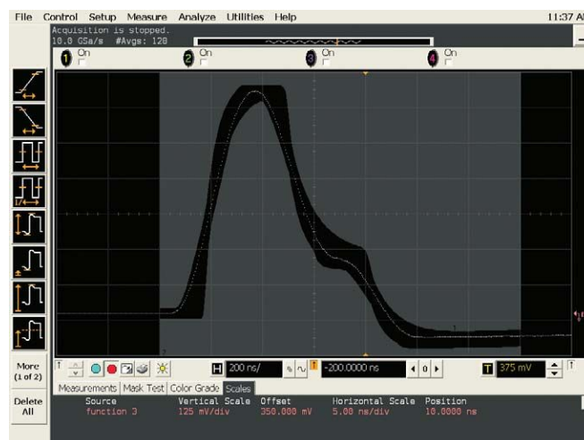
Figure 14c. The filtered and normalized point A waveform is then aligned to best fit to the template.
