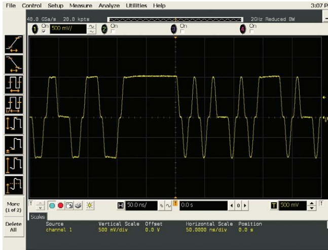
Figure 11. The MLT-3 coded idle pattern from a 100BASE-TX transmitter.
