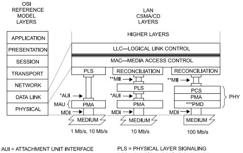
AUI = ATTACHMENT UNIT INTERFACE MDI = MEDIUM DEPENDENT INTERFACE MII = MEDIA INDEPENDENT INTERFACE MAU = MEDIUM ATTACHMENT UNIT PLS = PHYSICAL LAYER SIGNALING PCS = PHYSICAL CODING SUBLAYER PMA = PHYSICAL MEDIUM ATTACHMENT PHY = PHYSICAL LAYER DEVICE PMD = PHYSICAL MEDIUM DEPENDENT
