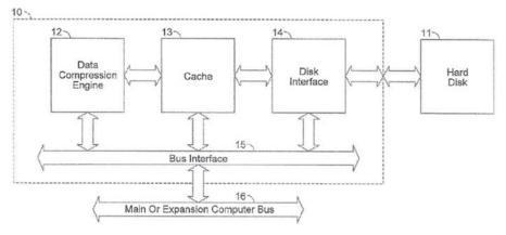
As shown in Figure 1, data storage controller 10 is "operatively connected" to hard disk 11 and to host system's bus 16. *Id.* at 5:63–6:53. Controller 10 includes cache 13 for data storage/preloading, and data compression engine 12 for data compression/decompression. *Id.* at 5:63–6:53, 20:50–22:11. The '862 Patent explains that, following reset or power on of a computer
