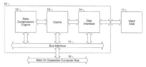
As shown in Figure 1, data storage controller 10 is "operatively connected" to hard disk 11 and to host system's bus 16. *Id.* at 5:63–6:53. Controller 10 includes cache 13 for data storage/preloading, and data compression engine 12 for data compression/decompression. *Id.* at 5:63–6:53, 20:50–22:11. The '862 Patent explains that, following reset or power on of a computer
