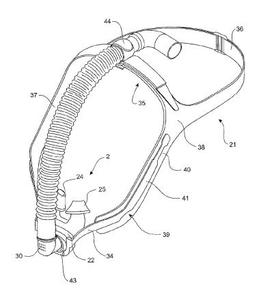
(57) Abstract: Headgear for use with a respiratory mask is described. The headgear comprises a continuous and substantially curved elongate member extending in use below a user's nose and at least two headgear straps capable of attachment to the ends of the elongate member. A mask attachment on the elongate member is disposed to sit below or on one of said user's nose, mouth, upper lip and an inlet to the mask. The attachment is capable of receiving the mask.
