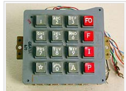
The keypads on telephones for the Autovon systems used all 16 DTMF signals. The red keys in the fourth column produce the A, B, C, and D DTMF events.
