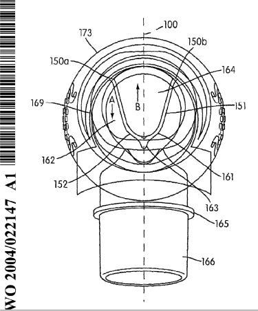
(57) Abstract: An elbow assembly for use in a respiratory mask, which includes an elbow, (160), an inlet port (162), an exhaust port (164) and a baffle (161) separating the inlet port from the exhaust port. A mask assembly includes a cushion (30) comprising at least one gusset and an aperture (42) for connection to the elbow assembly (20).
