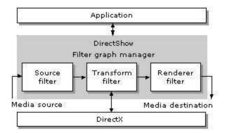
For example, the Microsoft MPEG filter graph uses the following filters.
