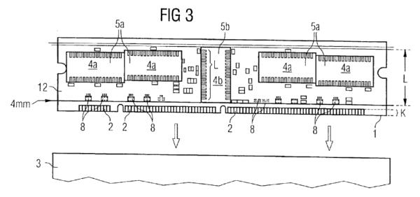
Figure 3 shows the rear side of a printed circuit board according to an embodiment of the '414 patent. *Id.* at 5:13–14. In this arrangement, housings 5a of semiconductor memories 4a are arranged horizontally on printed circuit board 1, and only housing 5b of error correction chip 4b is arranged vertically. *Id.* at 6:19–28. Housing 5b is "brought up to [] contact
