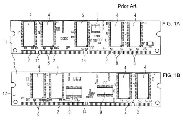
Figure 1A shows the front side of a conventional printed circuit board and Figure 1B shows the rear side of a conventional printed circuit board. *Id.* at 5:6–10. In a conventional arrangement, semiconductor memories 4 are arranged on the front and rear sides of the printed circuit board in the same orientation as error correction chip 5. *Id.* at 1:62–67. "In the case of this
