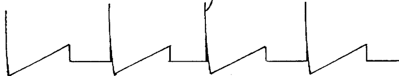
CURRENT IN POWER SWITCH 110
