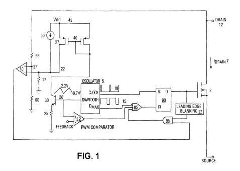
Figure 1 illustrates an embodiment of a power supply regulator circuit described in the '605 patent. Clock signal 10 sets latch 90 to enable power MOSFET 2 (i.e., turn the switch on). Ex. 1001, 4:19–24. Power MOSFET 2 is disabled (i.e., the switch is turned off) when latch 90 is reset by any one of three inputs to OR gate 85. *Id.* at 4:24–53. First,
