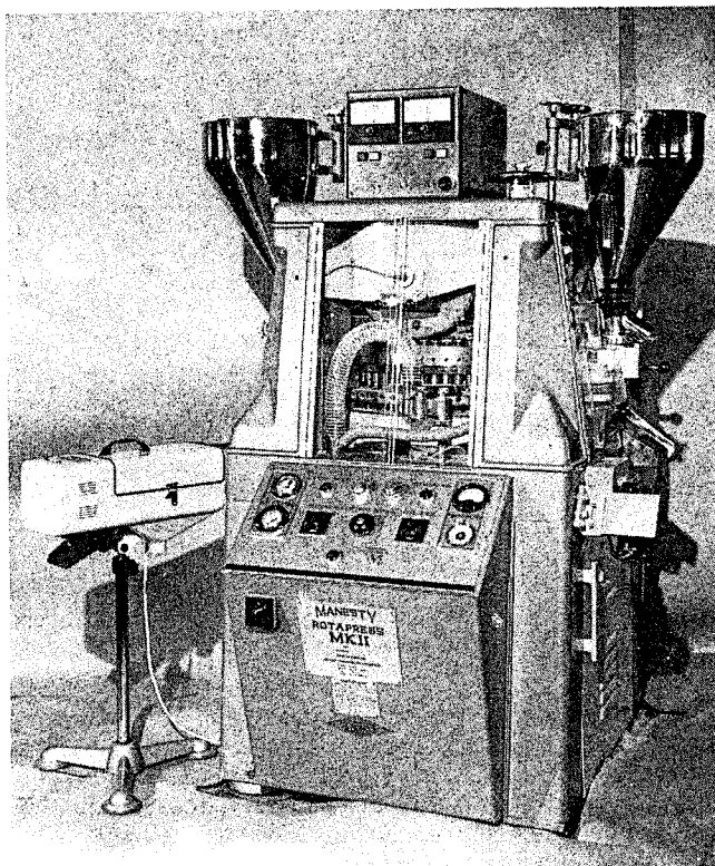
Fig. 89-26. Mark II Rotapress with 61 stations, equipped with deduster (left) and the Thomas Tablet Sentinel (top of press) (courtesy, Thomas/Manesty).
