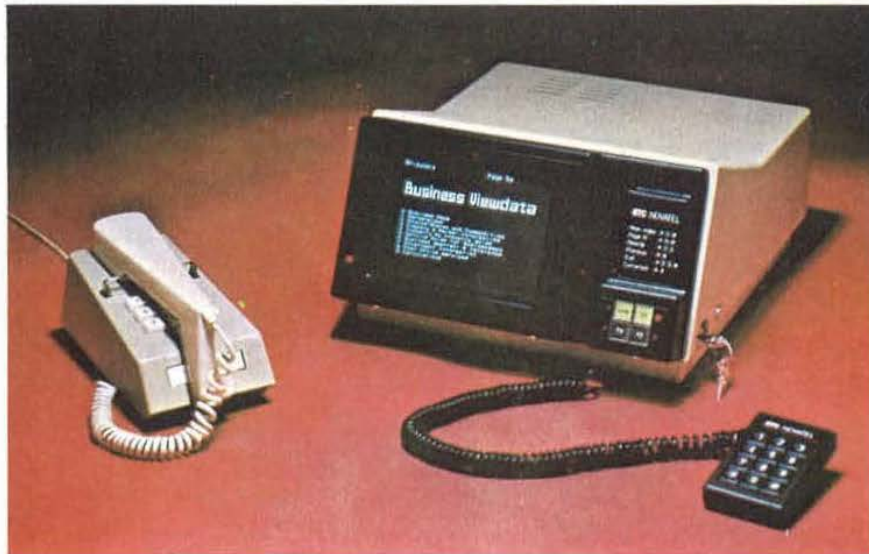
Figure 8.2. Typical business TV terminal.
