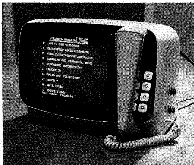
Office version of a Viewdata terminal, known as Viewdataphone. Note the integral keypad and telephone handset.
