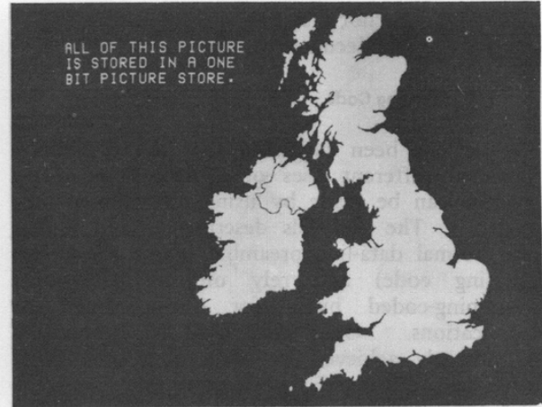
Fig. 5 - Example of picture-element resolution
