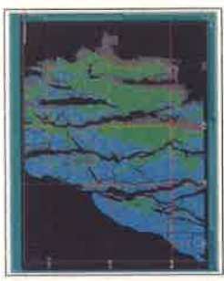
5. An example of fluid mapping from the North Sea Gullfaks field, uses data acquired and processed by Geco-Prakla. (Image courtesy of Statoil.)
