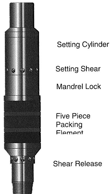
Figure 4 - The solid body packer is hydraulic set instead of inflatable (Guiberson / Halliburton Wizard II packer shown)
