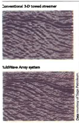
7. The section on the top shows data used in the North Sea using conventional towed streamers. There is a striking improvement in P-wave data quality gained from the MultiWave Array system (bottom). The target depth is approximately 3.5 km.
