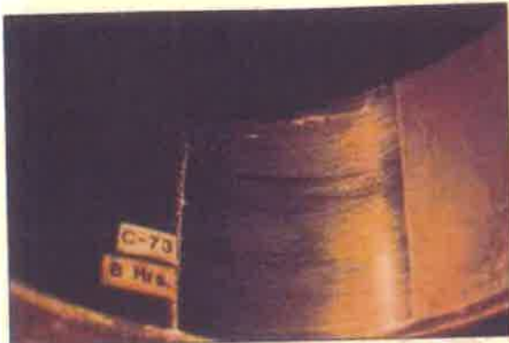
Fig. 6. The casing wear groove generated by a test is similar to those observed in the field.
