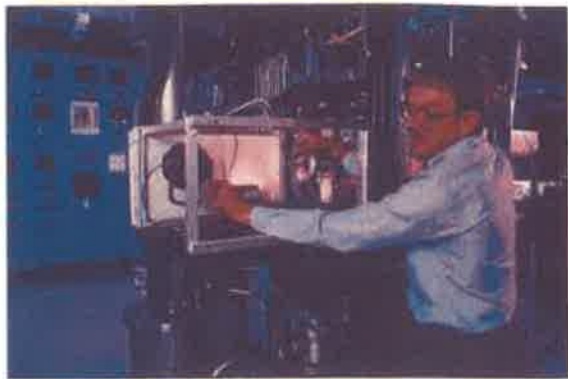
Fig. 1. Dr. Keith A. Truesdell of the Air Force Research Laboratory's Directed Energy Directorate works on a Chemical Oxygen-Iodine Laser (COIL). This laser technology was used aboard the Airborne Laser.
