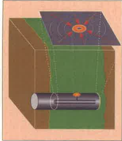
Fig. 5. Flow restricted by a probe on a wellbore is created in semihemispherical domain.
