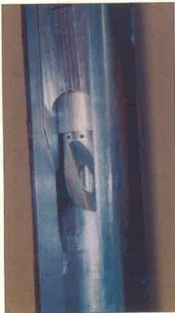
Fig. 1. The coiled tubing is deployed through a tubing diverter in the casing window.
