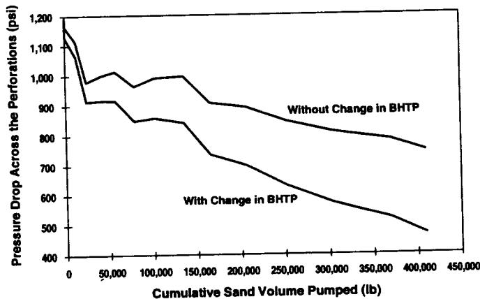
Fig. 2— $P_{perf}$  calculated with and without the change in BHTP.
