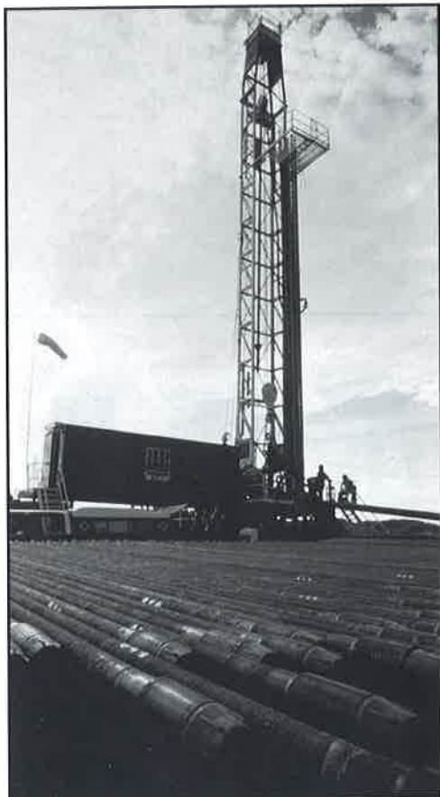
Figure 165. A completion rig running tubing into a well
