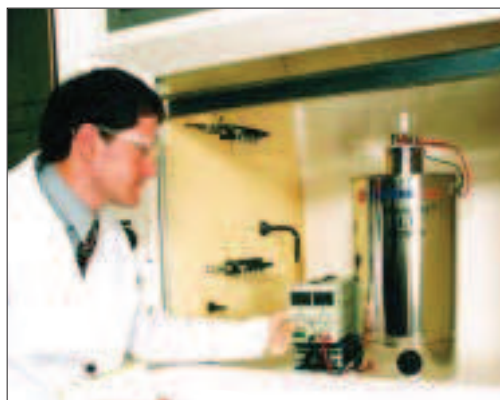
Figure 4. Laboratory-scale use of fluorine using the Fluorodec® LT generator (reproduced by permission of Fluorogas Ltd).
