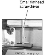
5. Place CR2032 Coin Cell Battery with plus (+) side up in the battery holder as shown.
