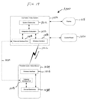
Figure 19 illustrates an embodiment of the disclosed system that provides wireless integration between car audio/video system 1010 and portable device 1024 in which integration subsystem 1032 is positioned within the car system. *Id.* at 8:3–8, 35:17–32. Wireless interface 1016 in the car system and wireless interface 1026 in the portable device form wireless link 1022. *Id.* at 34:15–18; *see id.* at 35:21–23.
