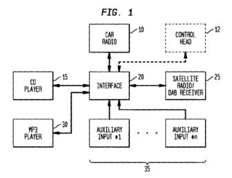
Figure 1 illustrates an embodiment integrating a CD player, a MP3 player, and a satellite radio or DAB receiver, and a number of auxiliary input sources with a car stereo. Ex. 1001, 3:12–13. As shown in the above figures, central to the '786 patent is an "interface" positioned between the car stereo and the audio device(s) and auxiliary input(s) being integrated.
