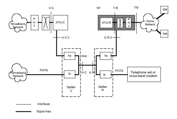
Figure 1 ADSL Forum System Reference Model
