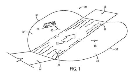
Figure 1 illustrates an embodiment of the half-pipe water ride with waterdelivery section 12, activity section 14, and dewatering section 16; activity section 14 includes middle section 34 and sidewalls 23. *Id.* at Fig. 1, 1:41– 42, 2:42–62, 3:22–24. Water from the dewatering section is returned to the water-delivery section through a water-retrieval section, as depicted in the embodiment of Figure 5. Figure 5 is reproduced below:
