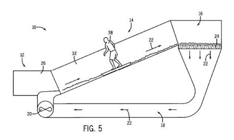
Figure 5 illustrates a cross-sectional view with pump 20 circulating water through a nozzle assembly and into the ride as described above. *Id.* at 1:49–50, 2:46–48, 2:58–62, 2:67–3:2.
