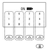
Each time you press the Select button (a), the Selection rectangle moves to another row (cycling through the three rows in turn). The Column buttons (a) each represent one of the four lines or programmable/intercom/drop buttons *in the row enclosed by the Selection rectangle*.
