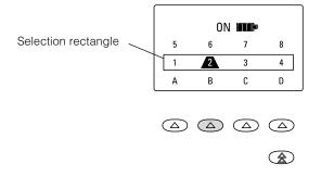
For example, suppose your handset shows the Selection rectangle around the middle row of lines. If you press the second Column button from the left (shaded in the illustration above), you select Line 2, as indicated by the truncated triangle in the illustration.
