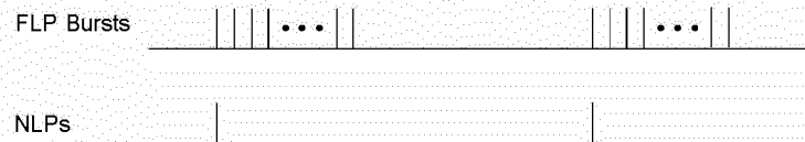
Figure 28-3—FLP Burst sequence to NLP sequence mapping
