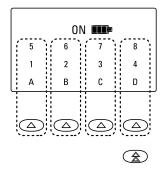
Each time you press the Select button ((1), the Selection rectangle moves to another row (cycling through the three rows in turn). The Column buttons ((2)) each represent one of the four lines or programmable/intercom/drop buttons in the row enclosed by the Selection rectangle.
