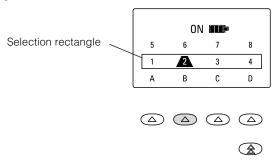
For example, suppose your handset shows the Selection rectangle around the middle row of lines. If you press the second Column button from the left (shaded in the illustration above), you select Line 2, as indicated by the truncated triangle in the illustration.
