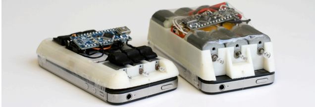
Figure 2: Our pocketOuija, here two versions of it, actuate the user's finger by moving a clear foil on top of the device's touchscreen (here an iPhone).
