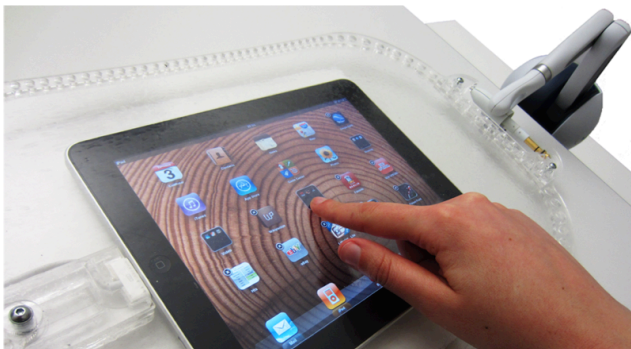
Figure 4: The longRangeOuija translates the user's finger via a clear foil actuated by a PHANToM arm.
