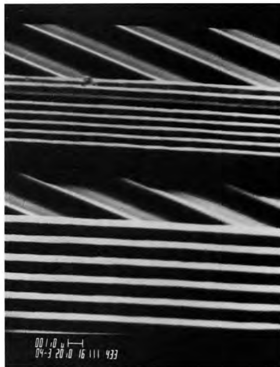
FIG. 10. (a) 1.0 \mu\text{m} lines and spaces in thick resist, using x ray for the top layer. The lines are traversing a 1.0 \mu\text{m} high, periodic grating to demonstrate good step coverage with no linewidth variation over steps (SEM photo). (b) Profile of the wall of resist for one of the 1.0 \mu\text{m} lines showing conformal coating of the wafer topology at the resist bottom and a flat surface at its top (SEM photo).
