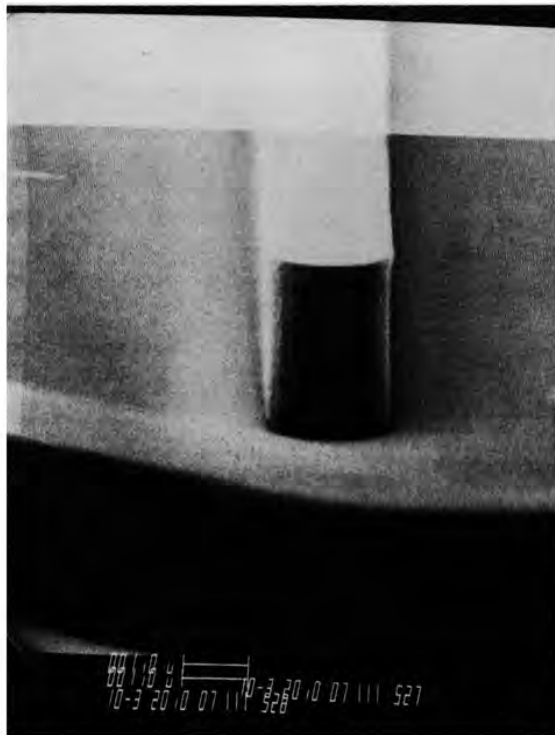
FIG. 7. Thick resist pattern obtained using optical patterning on a Perkin-Elmer projection printer for the top layer. (SEM photo).
