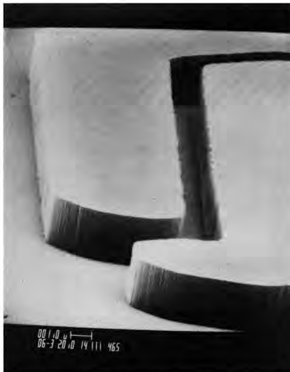
FIG. 5. Resulting pattern, which is all thick HPR resist, after using the trilevel processing described in Fig. 4. Top pattern was done with x-ray resist. The walls are 90^\circ and there is no linewidth loss (SEM photo).
