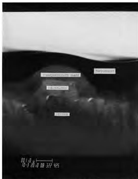
FIG. 1. X-ray resist thickness variation as it step covers 1.0\ \mu\text{m} of p -glass flowed over a 1.0\ \mu\text{m} high poly-silicon feature. Resist varies from 0.8\ \mu\text{m} on top of the feature to 1.7\ \mu\text{m} in the valley between features (SEM profile photo).
