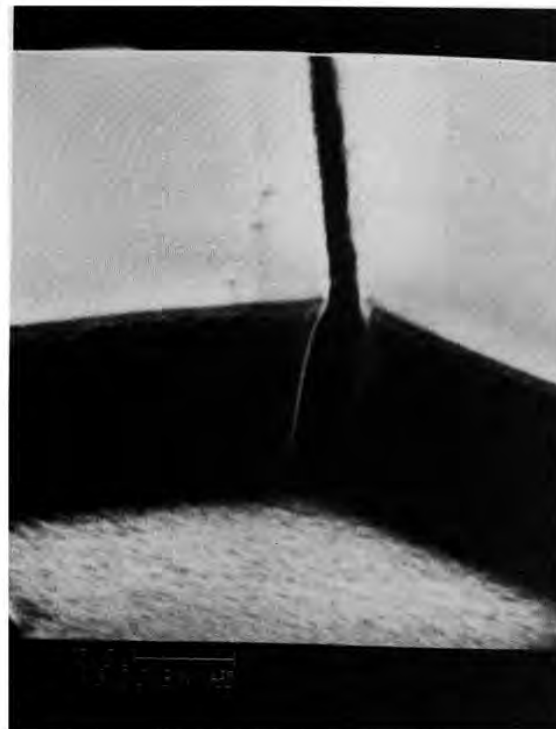
FIG. 8. Submicron trench for a Ga As gate obtained using a Kasper 10:1 step and repeat camera for the top layer. (SEM photo).
