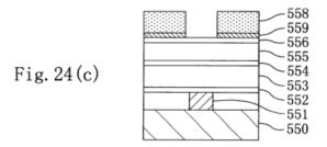
Figure 24(c), reproduced above, is a cross-sectional view of a partially-formed interconnection structure during a process step for forming the same. Ex. 1001, 9:28–31. In this step, titanium nitride film 557 is dry-etched using first resist pattern 558 as a mask, thereby forming mask pattern 559. *Id.* at 25:21–23.
