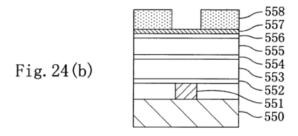
Figure 24(b), reproduced above, is a cross-sectional view of a partially-formed interconnection structure during a process step for forming the same. *Id.* at 9:28–31. In this step, first resist pattern 558 is formed on titanium nitride film 557. *Id.* at 25:19–21. First resist pattern 558 includes openings for forming wiring grooves of the interconnection structure. *Id.*
